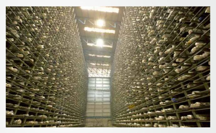
FeHR honeycomb warehousing system is completely suitable for large quantities and high access speeds. This system is used for automatic storage and retrieval of Bright Bars and Profiles. FeHR Cassette Rack System makes the best use of the available space and allows swift movement of the material from the packaging area to the storage area and all that is made possible with the touch of a button.
